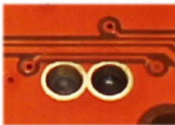
Figure 6 encoder LED and light sensor on bottom side of motherboard
