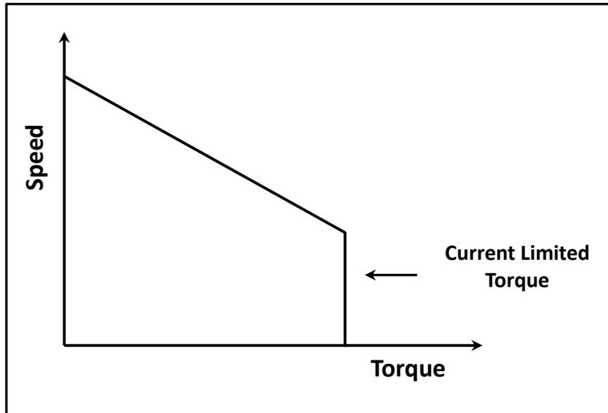
**Figure 4. Current Limited Torque**
