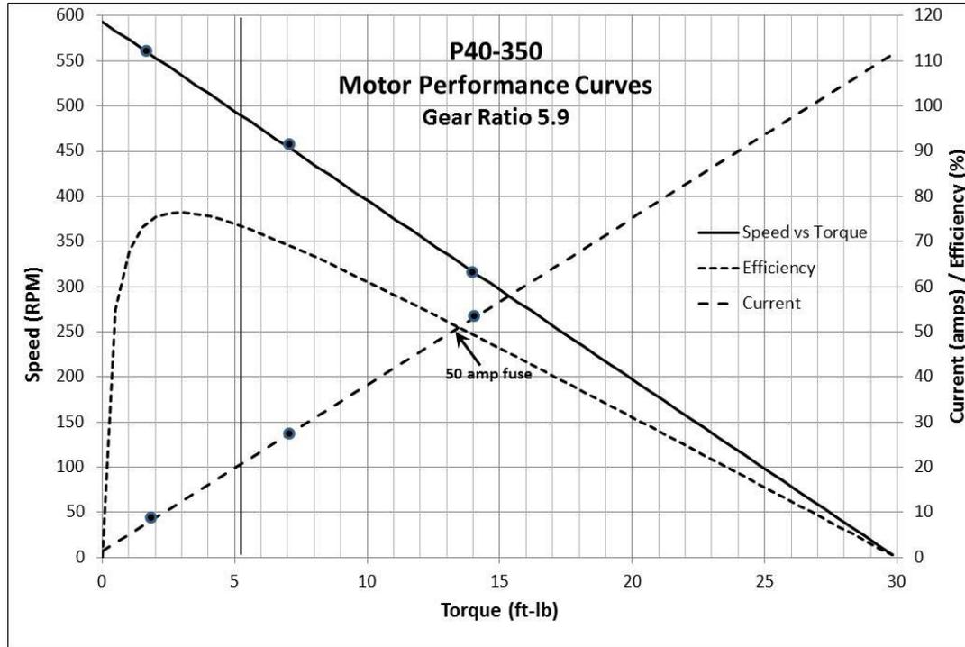
**Figure 6. Motor Performance: Gear Ratio 5.9**
