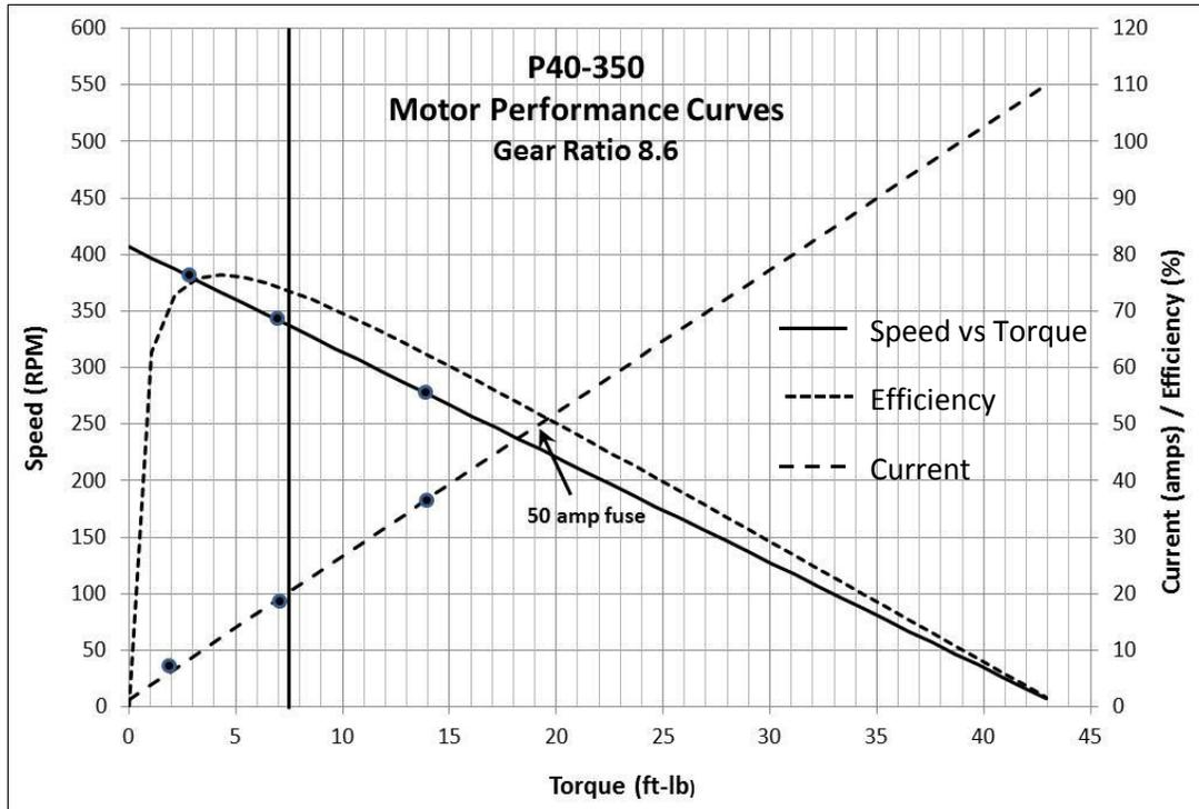
**Figure 7. Motor Performance Curve: Gear Ratio 8.6**
