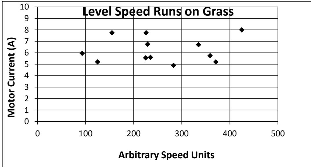
**Figure 9. Rover Motor Current vs. Speed**
