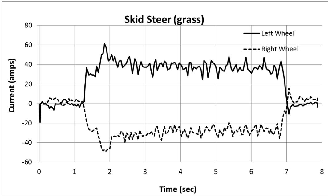
**Figure 10. Skid Steer Motor Currents**
