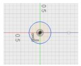
12. Use the **Sketch Dimension** tool to set the diameter of the circle to 0.25 inch. You have now completed the profile of the handle. Click on the **Stop Sketch** button.
