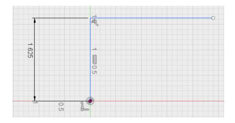
6. Use the **Sketch Dimension** tool to make the horizontal line 7.00 inches long.
