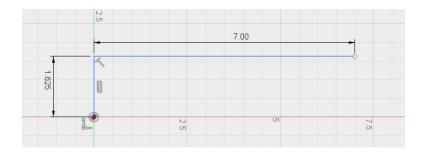
7. Draw a vertical line like the one illustrated below. The top end of the line should be coincident with the end-point of the horizontal line and the bottom end should be coincident with the horizontal axis line (red line). You now have the general outline of the sweep path for the handle. However, the path must be curved at each intersection of a vertical line with the horizontal line.
