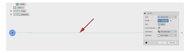
14. You should now have the 3-D object on your screen as illustrated below. You have created a 3-D object with the Sweep tool! Click on the **OK** button in the SWEEP dialog box to complete the operation.
