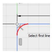
9. A dimension box should appear on screen as illustrated below. Enter a value of 0.75 to make the radius of the fillet 0.75 inches. Then press the Enter key to set that value. Repeat this procedure for the other corner.
