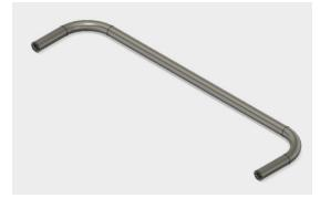
You will be creating a drawer handle like the one illustrated to the left. The procedure requires the drawing of two sketches: 1) a sketch of the path for the sweep and 2) a sketch of the cross section of the handle, which is a circle. The image below provides the dimensions of the handle. Note that the ends of the handle have threaded holes to accommodate screws.
