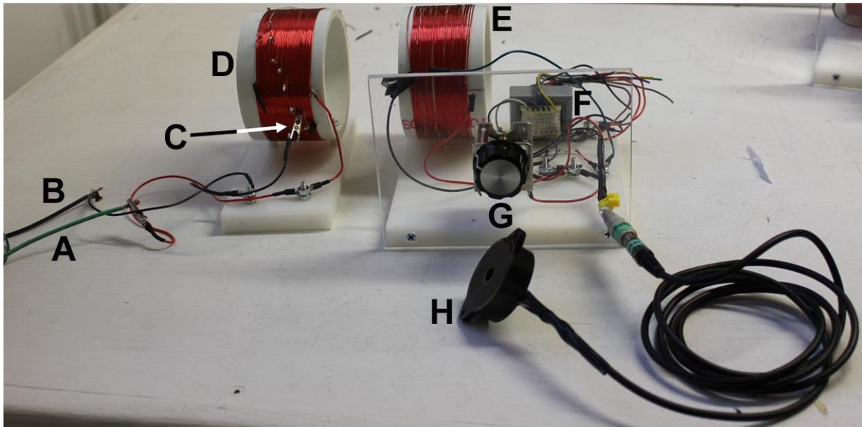
Figure 4 assembled crystal radio
