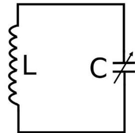
Figure 5 simple LC circuit with coil and variable capacitor
